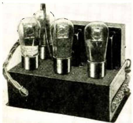
Fig. B Photograph of the amplifier itself. The cable connects to the batteries housed in the case.
